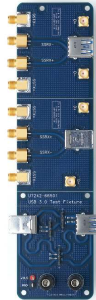
Figure 5. The Keysight U7242A USB 3.0 transmitter and receiver compliance test fixture.
